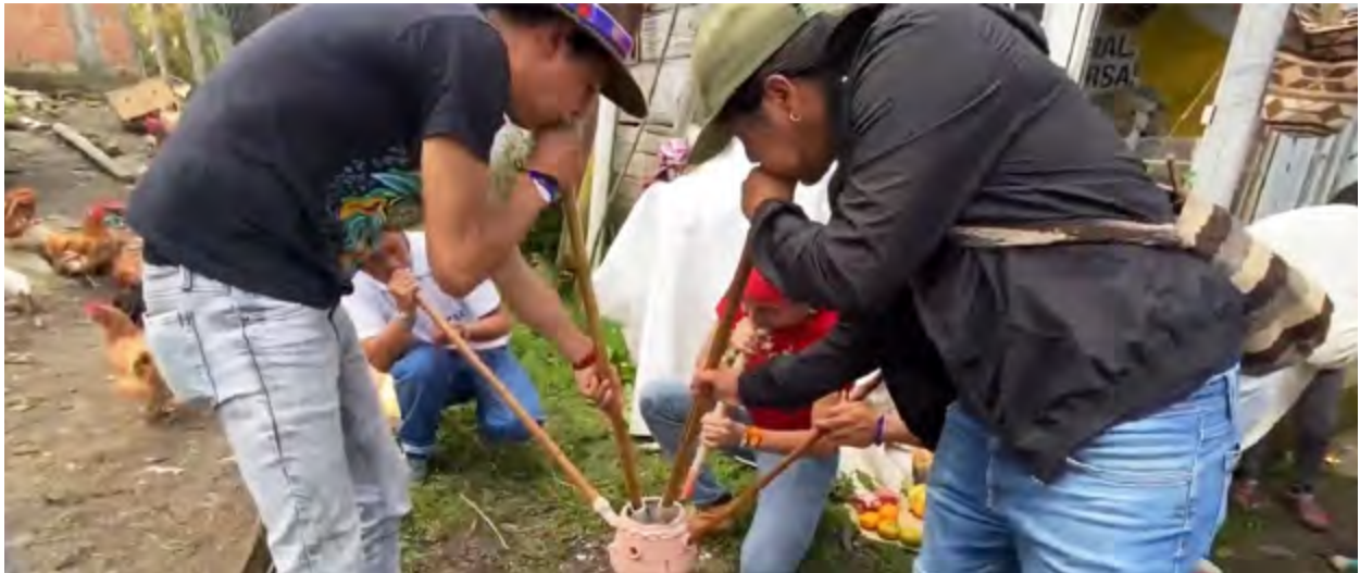
Blowing air into the kiln to reach the proper temperature. Photo credit: Jhon "La Gueba del Jhon" Rojas
